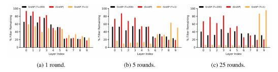
Figure 16: Layer-wise pruning ratios for VGG-13 with a target ratio of 65% pruning. Results are provided for pruning over (a) 1 round, (b) 5 rounds, and (c) 25 rounds. When the model is allowed to train even slightly, GraSP without temperature prunes earlier layers very aggressively.
